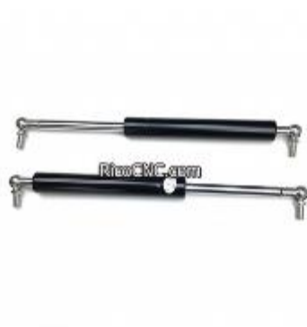
4-010-04-0092 4010040092 Gas Shock Absorber Type 16-6 stroke 115 L 365 1600 N for Homag KAL211
