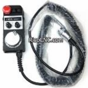
iHDW-BPACS-IM-C20 FUTURE Electronic Hand wheel Unit Generator
